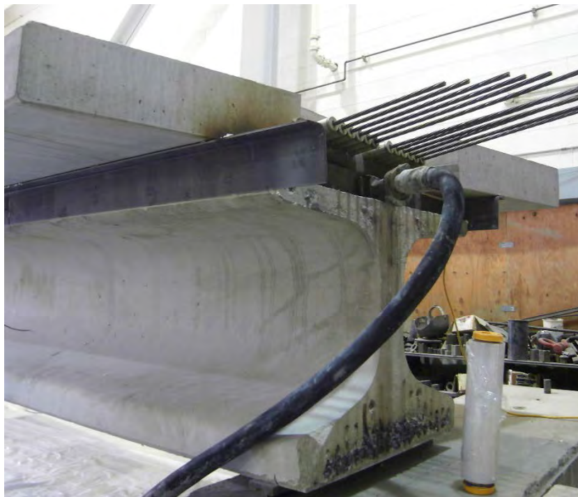
Figure 4.13 – Pumping concrete from the other end of the specimen
