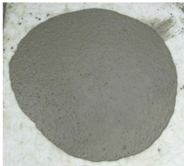
Figure 4.9 – Slump flow of the SCC mixture used in the pumping test (VSI = 0)
