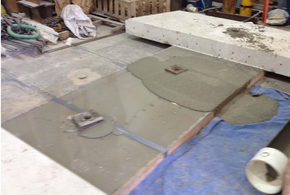
Figure 5.7 – Concrete overflowing at one of the joints between Plexiglass sheets
