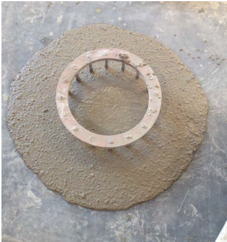
Figure 5.3 – Slump flow (top) and J-ring (bottom) tests (VSI = 0)
