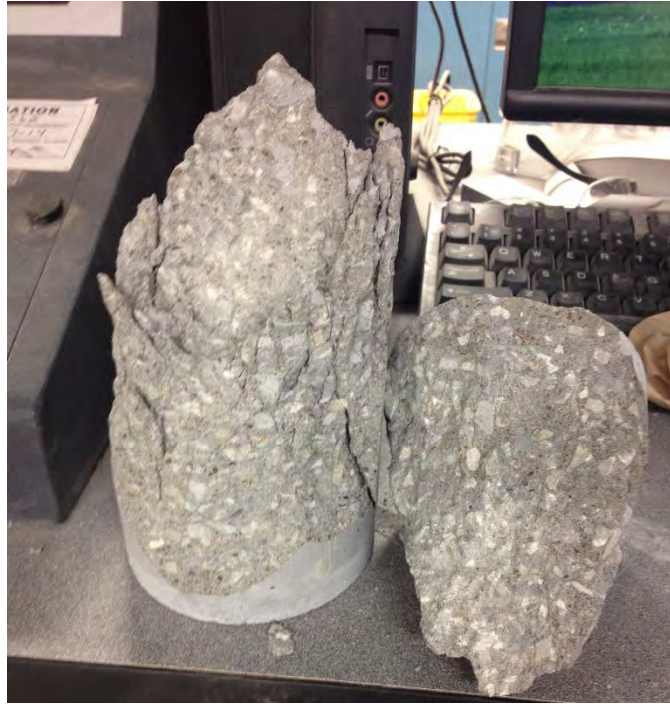
Figure 4.8 – Coarse aggregate distribution in joint concrete (HVSI = 1)
