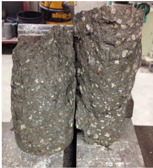
Figure 5.8 – Coarse aggregate distribution in hardened concrete (HVSI = 0)
