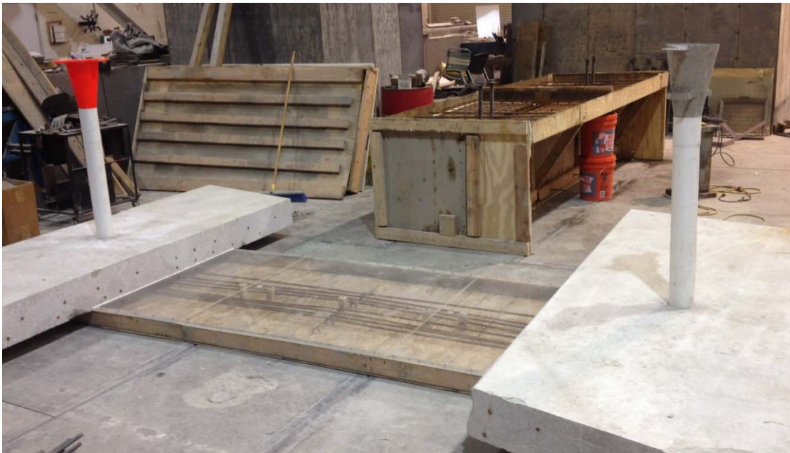
Figure 5.2 – Photos of the pouring mockup test specimen
