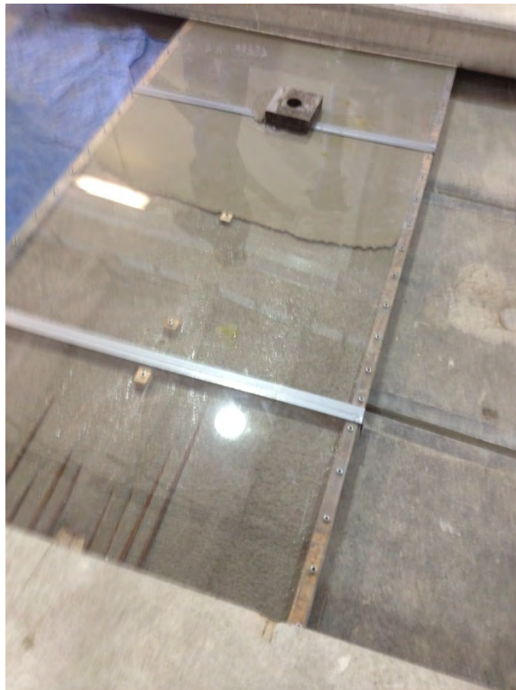
Figure 5.6 – SCC flowing from one port to the other and completely filling the channel
