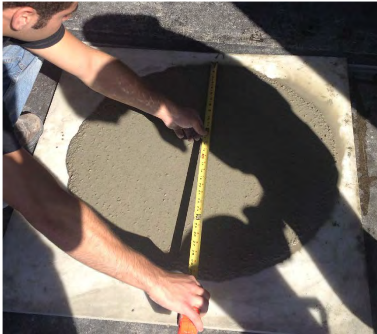
Figure 4.7 – Slump flow of the SCC mixture used in filling transverse joints (VSI = 1.0)
